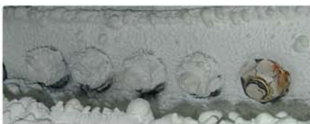
The difference between a wet coated system and a bolt cap system after a fire.
